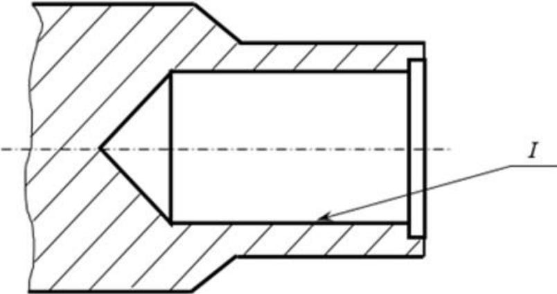
The drawing shows a technical drawing of a mechanical part. It consists of a cylindrical section on the right and a more complex, stepped section on the left. A horizontal dashed line represents the axis of symmetry. A line labeled 'I' points to a specific surface on the cylindrical part, indicating where a thread should be drawn.
